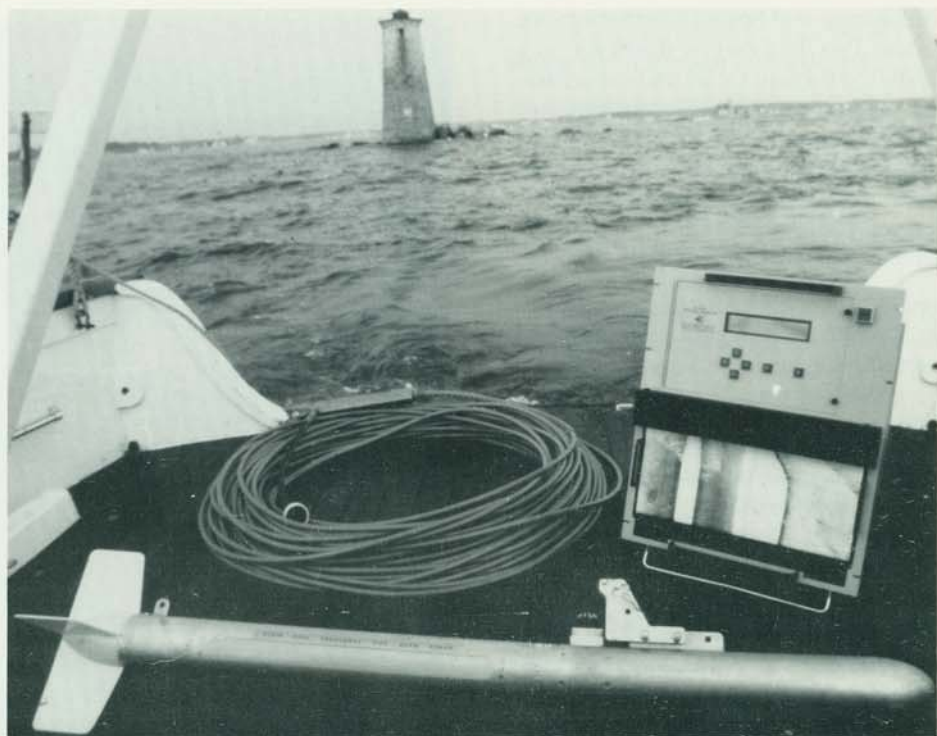
Photo 2 - Klein Lightweight Side Scan Sonar System consisting of 595 Digital Thermal Recorder and Simultaneous 100/500 KHZ Dual Frequency Towfish
