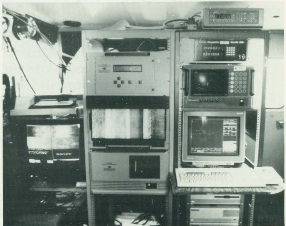
Photo 1 - Typical Integrated Side Scan Sonar System for MCM
